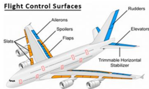
Flight Control Surface Testing LVDT/RVDT Simulation and Measurement
