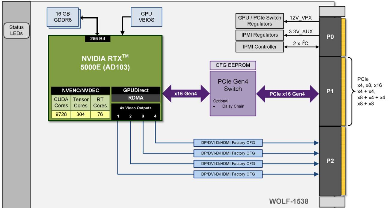
The SOSA Aligned HPC model supports slot profile 14.6.11 with up to PCIe Gen4 support.
