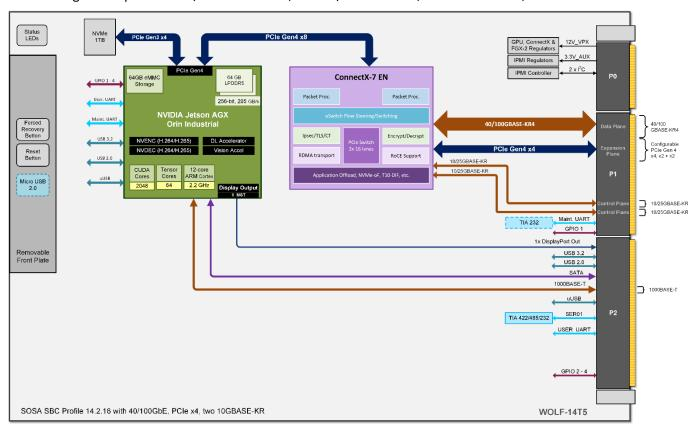
The following model provides two 10/25GBASE-KR, one 1000BASE-T and PCIe Gen4 x8
