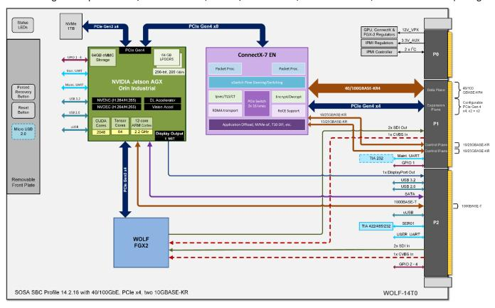
The following model provides two 10/25GBASE-KR, one 1000BASE-T and PCIe Gen4 x8 (configurable).
